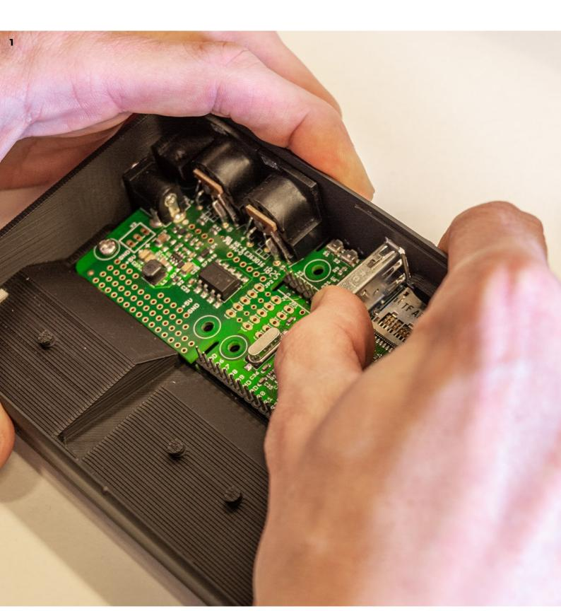
Use the two short M3 screws to complete the attachment of your Axoloti. You will need a cross-head screwdriver to do this step. Do not tighten the screws too much.
