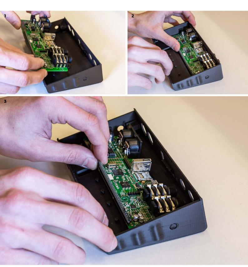
Push slightly the USB host port from the backside through the plastic space till you hear a "click".
